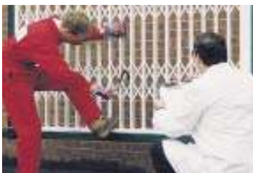
Citadel Plus undergoing a simulated attack test
