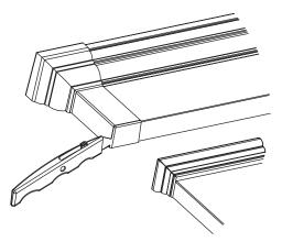
Place the Transition Top pieces on the Header in the approximate locations of the Pilasters. If the Header has the optional Endcaps welded on, use a utility knife to trim the bottom of the Endcaps so that the Transition Top pieces are flush. See figure at left. Clip them to the header using the clips provided. Use two clips per Transition Top. See figure below.
